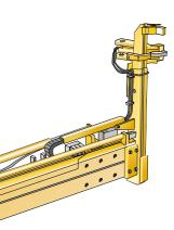
side corner castings of both containers. In addition to the side clamps position monitoring, a combination of mechanical sensing pins and electrical container detection sensors ensure maximum safety during handling operation, either with one or two containers.
